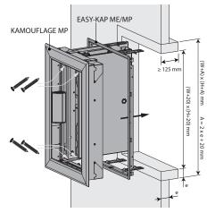
1. Coat the edges of the opening with adhesive plaster, type FACILIS.
