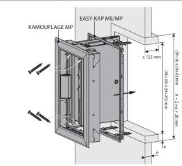
1. Put glue type CF GLUE on the uprights and cross pieces and between the lining and the wall. Screw the sleeve using chipboard screws Ø5 x 70 mm at 150 mm intervals. Two fixing lugs are provided at the bottom and at the top of the mounting frame: fold these against the sleeve. First coat the opening with glue CF GLUE. Glue the mounting frame to the lining taking care not to misshape it. The finished opening must have the same size as the mounting frame (W+10) x (H+10) mm.
