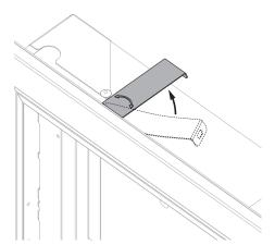
1. Rotate the four fastening plates on the damper  $90^{\circ}$  (to the upright position).
