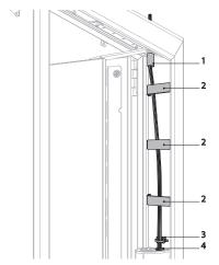
4. Lead the cables through the opening. Use the protective sleeve (1), the fixation clips (2) and the plastic cable clamp (3) to attach the cables to the frame. Lead the cables to the connection box through the grommet (4) and connect according to the electrical connection diagram.
