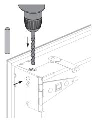
2. Drill a hole in the refractory material at the chosen corner(s). The galvanised part at the inside of the shutter is already indented.
