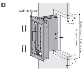
1. Assemble the sleeve with staples and affix the assembled sleeve to the duct wall with staples.
