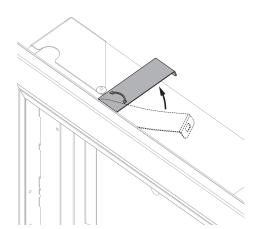
1. Rotate the four fastening plates on the damper  $90^{\circ}$  (to the upright position).
