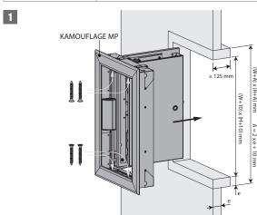
1. Coat the edges of the opening with adhesive plaster. Seal the joints between uprights and cross pieces and between the lining and the wall with vegetable fibre caulking and plaster.
