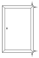
1. The electrical connection is possible via the 2 corners at the side of the hinges.
