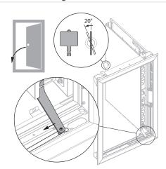
1. Turn the key 20° anti-clockwise. Push the actuating arm in the direction of the arrow and pull the shutter into its closed position.
