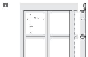
2. In case several shutters are mounted at a minimal distance, the bearing and reinforcement points of the duct must be adjusted in proportion to the increased weight. The installation of the duct must comply with the classification report delivered by the duct manufacturer.
