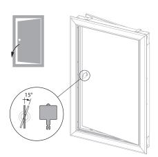
2. Turn the key 15° clockwise. The key blocks in the lock and the door can be pulled into its lock.
