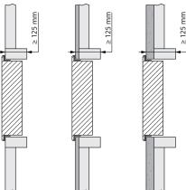
3. In order to prevent cracks around the opening in the long term, a finishing layer (plasterboard, (cellular) concrete, rigid wall) can be added between the mounting frame and the opening.
