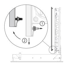
1. The ATOUT option facilitates the finishing of the shutter. You can remove the front plate by unscrewing the bolts at the bottom and top on the hinge side. Then you can slide the plate in the direction of the hinges.
