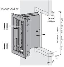
2. Make an opening with dimensions (W+A) x (H+A) mm. A = 2 x thickness sleeve (e) + 10 mm.
