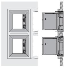
1. The shutters can be installed at minimal distance on top of or next to each other, if they are mounted in separate sleeves made from the duct material with the required fire resistance. It is advised not to exceed a 4 x 2 configuration (W x H).
