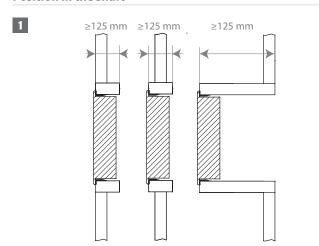
1. The shutter is affixed to the smoke control duct through a sleeve. That sleeve can be installed either in the duct, in the axis of the duct or outside the duct (or duct extension).
