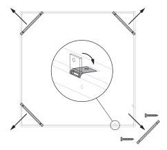
3. Put aside the screws that are affixed to one of the cross slats, then unscrew the 4 cross slats of the mounting frame and fold the 8 fastening plates in the frame.
