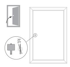
2. Unlocking 1V Turn the key 20° anti-clockwise and push the shutter into its open position.
