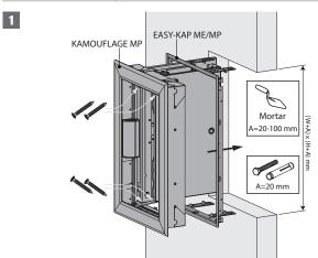
1. In case the mounting frame is screwed: Make an opening with dimensions (W+20)  $\times$  (H+20) mm. In case the mounting frame is fixed with mortar: Make an opening with dimensions (W+20)  $\times$  (H+20) mm till (W+100)  $\times$  (H+100) mm.
