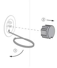
1. Remove the finishing cap from the shutter. To do this, use the hook with key ring that is delivered with the product. You may attach this tool to the key through its handy key ring.
