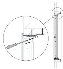
5. Open the shutter and position it in the mounting frame. Fasten the shutter onto the mounting frame with the 4 screws supplied, as shown in the drawing. Tightening the screws pulls the shutter towards the wall until its final position. You can also slightly correct the angle of the shutter with respect to the mounting frame.
