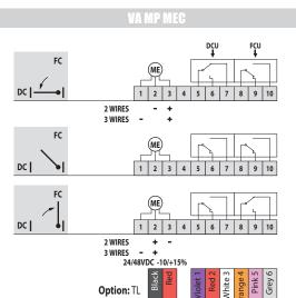
**DC:** Switch closed position smoke evacuation shutter **FC:** Switch open position smoke evacuation shutter
