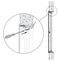
5. Open the shutter and position it in the mounting frame. Fasten the shutter onto the mounting frame with the 4 screws supplied, as shown in the drawing. Tightening the screws pulls the shutter towards the wall until its final position.
