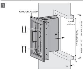
1. Put glue type CF GLUE on the uprights and cross pieces and between the lining and the wall. Screw the sleeve using chipboard screws  $\emptyset$ 5 x 70 mm at 150 mm intervals.
