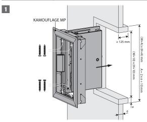
1. Put glue type GLASROC F V500 on the uprights and cross pieces and between the lining and the wall. Screw the sleeve using chipboard screws Ø5 x 70 mm at 150 mm intervals.
