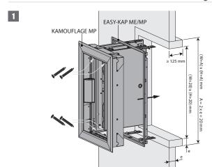
1. Make an opening with dimensions (W+A) x (H+A) mm. A = 2 x thickness sleeve (e) + 20 mm.
