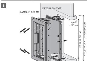
1. Assemble the sleeve with staples and affix the assembled sleeve to the duct wall with staples.
