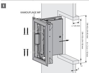
1. Coat the edges of the opening with adhesive plaster, type FACILIS.
