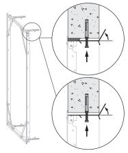
2. The mounting frame should always be fastened to the concrete shaft with screws and dowels (Ø 6 x minimum 60 mm, steel or stainless steel).
