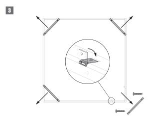
3. Put aside the screws that are affixed to one of the cross slats, then unscrew the 4 cross slats of the mounting frame and fold the 8 fastening plates in the frame.
