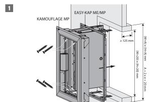
1. Coat the edges of the opening with adhesive plaster type PLACOL (in case of Geoflam) or GEOCOL (S) (in case of Geotec). In case of Geotec you can also assemble the sleeve with glue and screws  $\emptyset$  5 x (2 x e) mm and affix the assembled sleeve to the duct wall with glue and screws  $\emptyset$  5 x (2 x e) mm every 100 mm.
